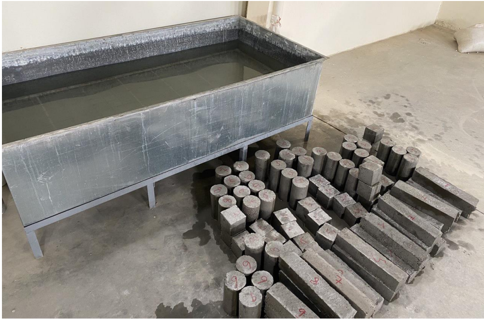
Fig. 5 Concrete specimens after curing
